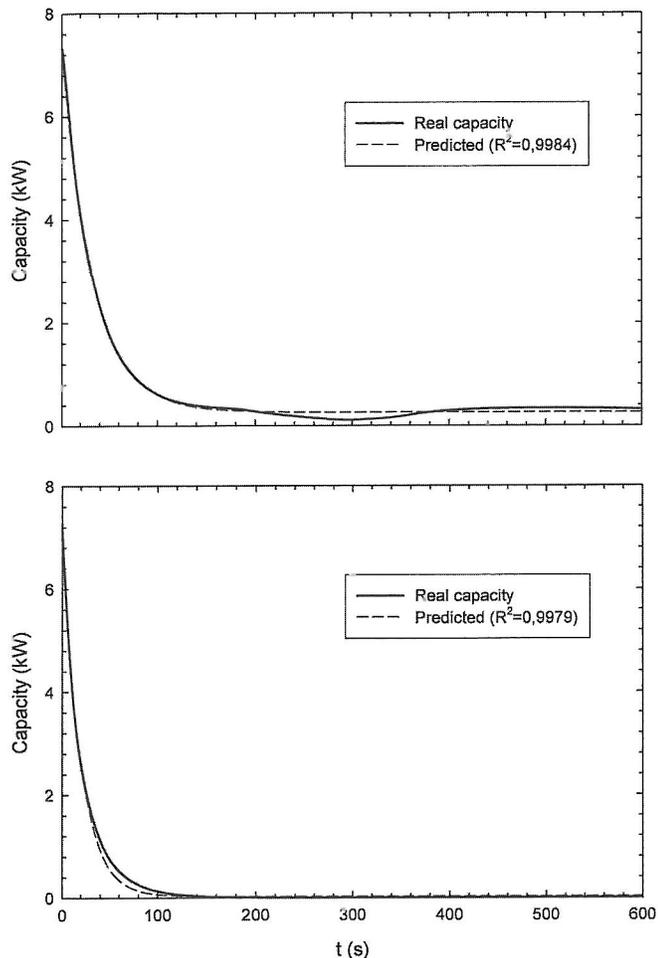
Figure 5 Modeling the variation of the capacity at compressor shutdown.
