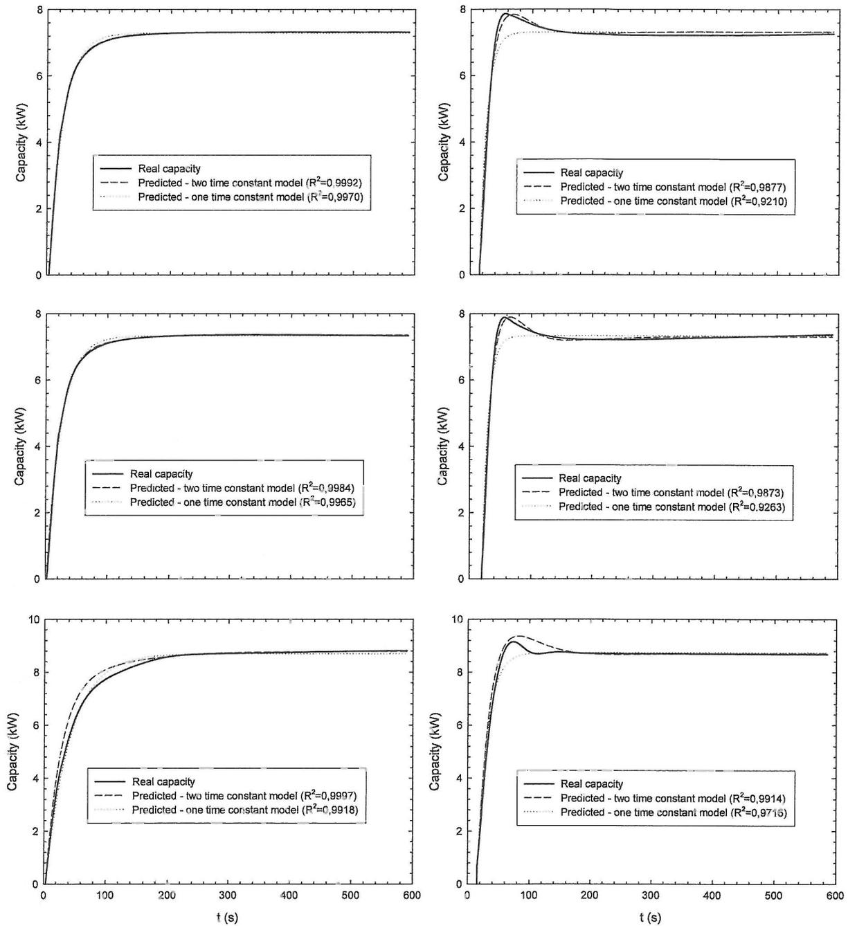
Figure 4 Modeling the variation of the capacity at compressor start-up.
