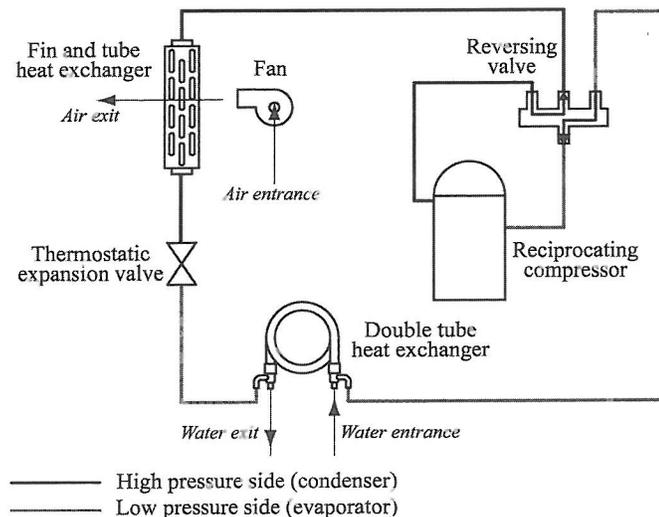
**Figure 1** Schematic representation of the modeled heat pump (shown in heating mode).
