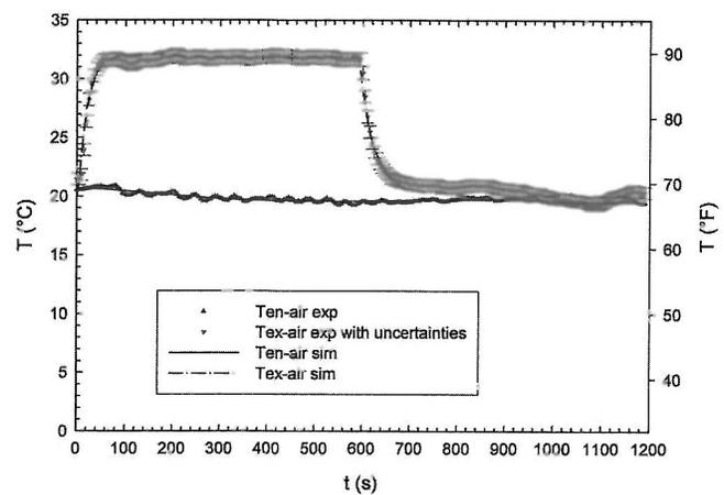
**Figure 2** Comparison between the model and experiments: variation of the outlet air temperature.
