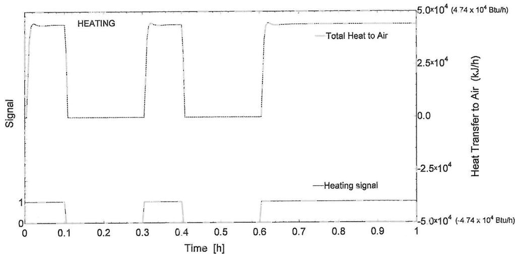
Figure 6 TRNSYS screen capture showing the response of TYPE 801 to a heating input signal.
