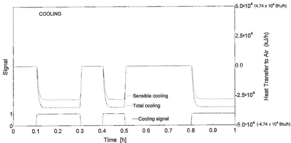
Figure 7 TRNSYS screen capture showing the response of TYPE 801 to a cooling input signal.
