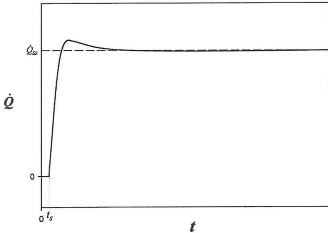
**Figure 3** General format of the variation of the capacity at compressor start-up.
