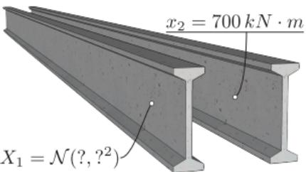
The prior knowledge of the resistance  $(X_1, X_2)$  for two adjacent beams is
