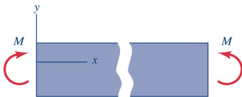
(a) Pure bending in longitudinal plane of symmetry.
